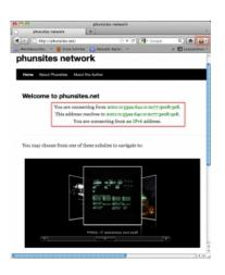
This will help you identify quickly which protocol the site is running. Klicking on the dropdown will reveal further information about the remote and local IP addresses.
