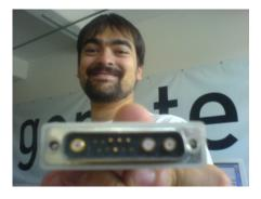
P.S. The modified adaptor would not work on a SUN aftwards. As stated earlier only one pin must really be broken off which possible allows dual-use of the adaptor on both SGI and SUN boxes. As to my knowledge two of the pins are looped to allow a SUN to detect a monitor. Since I didn't bother in going through the SUN tech sheets this is unverified information. If somebody out there knows it please drop me note.
